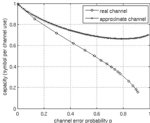
Fig. 2. Capacity of the real channel model and the approximate channel.
