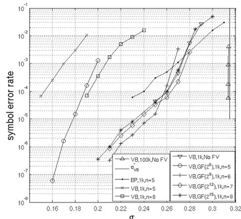
Fig. 3. Simulation results comparing the VB decoder with the full BP decoder using the real channel model.
