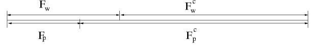
Fig. 2. Illustration of relationship between F_{\mathcal{W}} and F_{\mathcal{P}} . The line represents the indexes, and F_{\mathcal{W}} and F_{\mathcal{P}} are the frozen set for the WEM channel \mathcal{W} and the storage channel \mathcal{P} , respectively.
