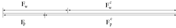
Fig. 2. Illustration of relationship between F_{\mathcal{W}} and F_{\mathcal{P}} . The line represents the indexes, and F_{\mathcal{W}} and F_{\mathcal{P}} are the frozen set for the WEM channel \mathcal{W} and the storage channel \mathcal{P} , respectively.
