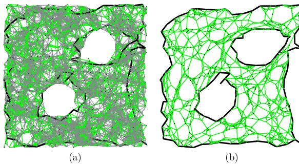
**Fig. 8** Wireless sensor network and its planarization. **(a)** The *black* (*darkest*) edges and the *green* (*darker*) edges are the planarized network. The *light* (*grey*) edges are the remaining edges in the original network. The original network is a quasi-UDG with  $N = 2000$  nodes and average degree 12, where transmission ranges vary by as much as  $R/r = 5$ . **(b)** A plane embedding of the planarized network
