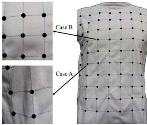
Fig. 5. Model of the clothes and the distance analyze of nodes: case A/case B is the loose/tight cloth and the distance between two adjacent nodes is less/large than the original distance.
