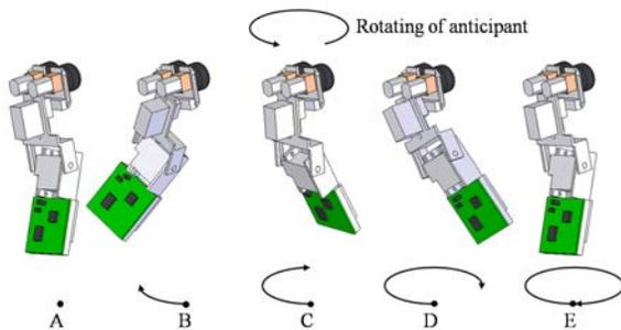
Fig. 10. Tail's motion to recover from a side tumbling
