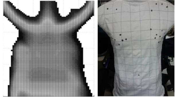
Fig. 11. Comparison between the model and the actual unreachable area: the black points on the clothes in the right figure are the recorded points where the robot cannot climb, while the white area in the left figure is the theoretical unreachable region. They have the similar shape on the clothes.
