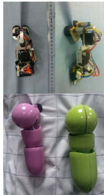
Fig. 1. Prototype and the improved versions of Clothbot: the upper figures are the prototype of Clothbot and the lower robots are the improved Clothbots, which are equipped with protective shells.
