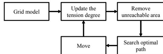
Fig. 4. Diagram of the path planning
