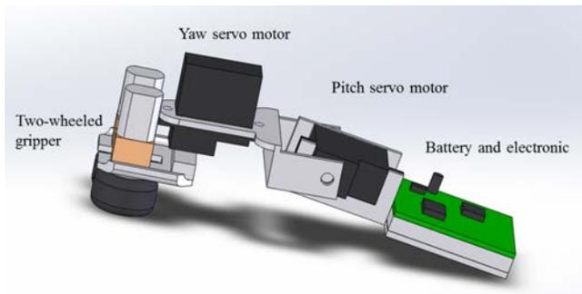
Fig. 2. Structure of Clothbot: Clothbot is composed of a two-wheeled gripper and a 2-DOF tail. The tail consists of the yaw and pitch servo motors. The battery and electronic are fixed at the end of the tail.
