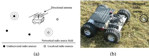
Fig. 1. (a) Schematics of deploying a single mobile robot to localize unknown networked radio sources. The radio sources with dashed circles indicate that they are sending radio signals. (b) A prototype of a mobile robot and a radio source.
