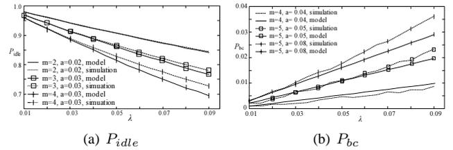
Fig. 6. Comparison of  $P_{idle}$  and  $P_{bc}$  from the network simulation and the proposed model under different values of  $a$ ,  $m$ , and  $\lambda$ .
