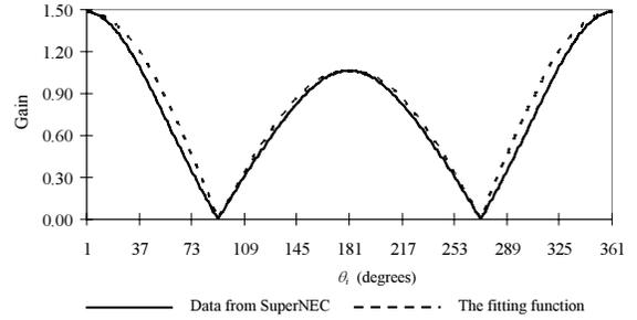
Fig. 4. LPDA antenna gain curve fitting.
