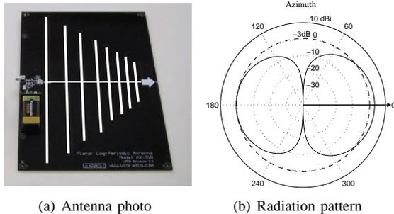
Fig. 3. WiNRADiO AX-31B planar log-periodic directional antenna properties.
