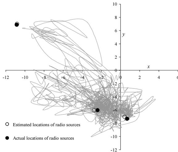
Fig. 8. Sample robot trajectory with network size  $m = 3$ .
