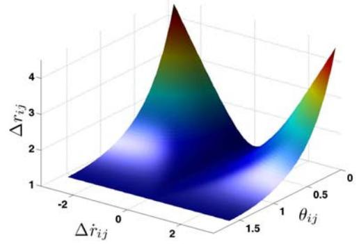
Figure 4. Surface of safety region  $X_{ij}^S$  in  $\mathbb{R}^2 \times S^1$  for a case of  $a_{\max}^{R_i} = 1$  m/s<sup>2</sup> and  $l_j = 1$  m/s for  $\theta_{ij} \in [0, \frac{\pi}{2}]$ .
