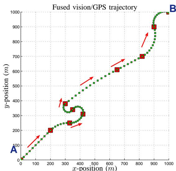
Fig. 2. An example of motorcycle trajectory from point A (with coordinates (0,0)) to point B (with coordinates (1000m,1000m)) (large red squares represent GPS waypoints and smaller green squares represent the fused vision/GPS target points).
