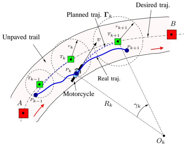
Fig. 4. A schematic of the vision/GPS motion planning.
