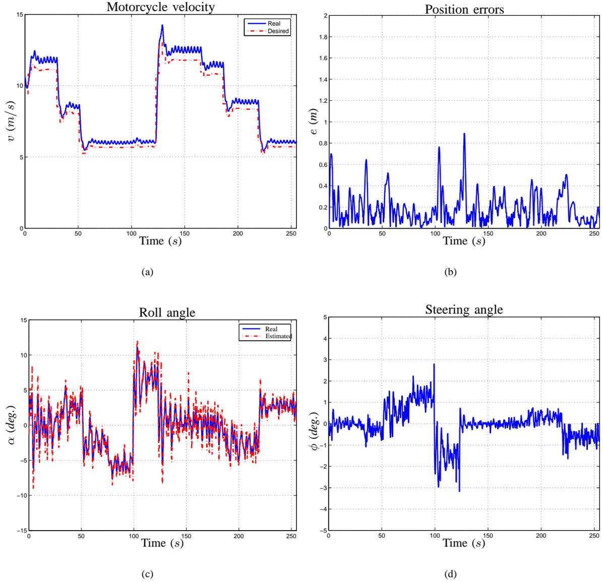
Fig. 6. Simulation results of the motorcycle trajectory tracking control with measurement noise. (a) velocity, (b) position error with center of the road, (c) roll angle  $\theta$ , (d) controlled steering angle  $\phi$ .
