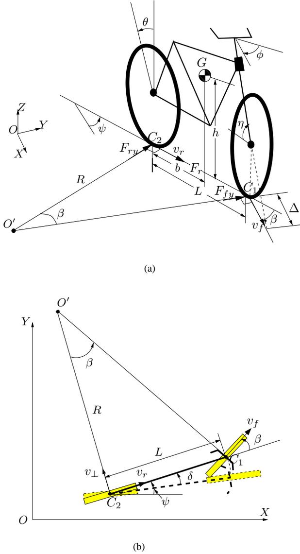
Fig. 1. A kinematic diagram of the motorcycle dynamics. (a) Schematic view of a motorcycle on a plane, (b) top-view of the motorcycle.
