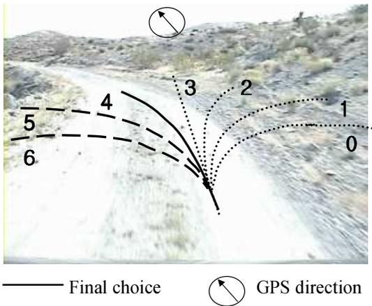
Fig. 3. An example of the fused GPS/vision direction output on an offroad trail in the desert. Dashed lines are candidate feasible trajectories from vision systems and the solid line is the final choice direction fused with GPS information.
