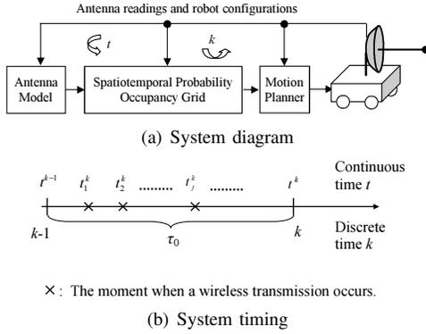
Fig. 2. An illustration of system diagram and timing.
