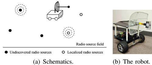
Fig. 1. Schematics of deploying a single mobile robot to localize unknown transient radio sources. The radio sources with dashed circles indicate that they are sending radio signals.
