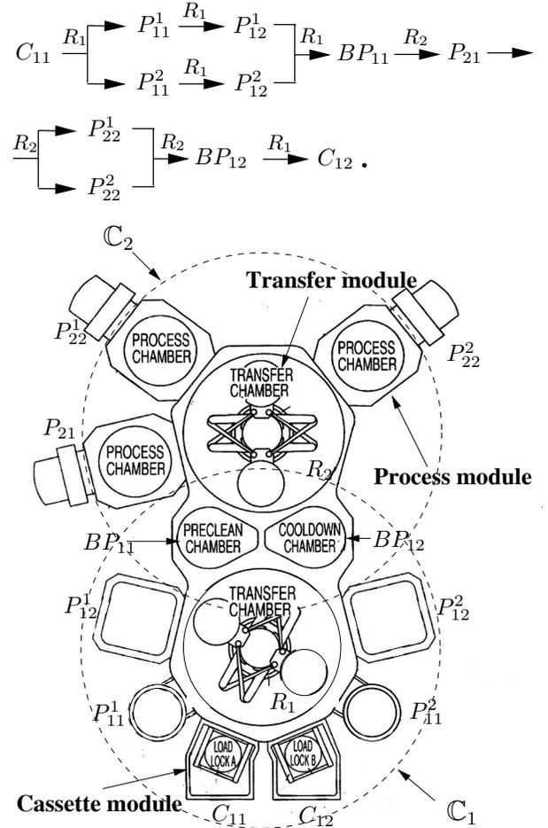
Fig. 5. A schematic layout of a CVD cluster tool.
