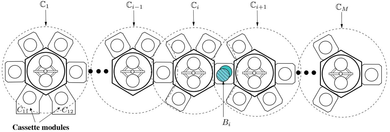
Fig. 2. A schematic of an inter-connected  $M$ -cluster tool.
