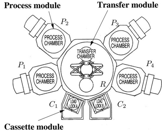
Fig. 1. A schematic of a cluster tool.
