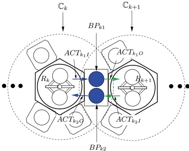
Fig. 3. A combined buffer/process module (BPM) with a two-wafer capacity.
