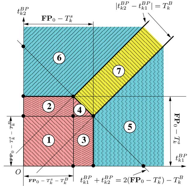
Fig. 4.  $\mathbf{FP}$  calculation for different BPM process times  $t_{k1}^{BP}$  and  $t_{k2}^{BP}$  if  $S_k = 2$ .
