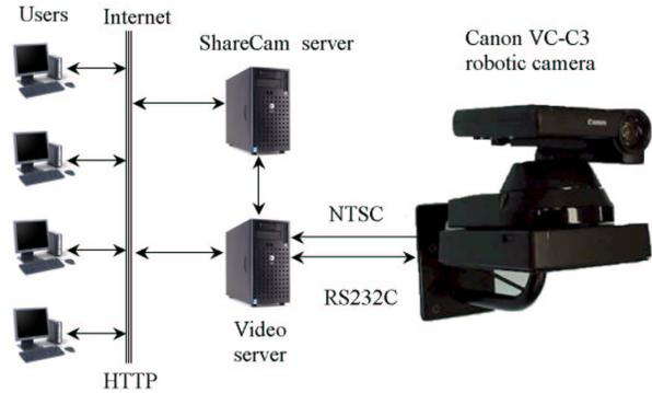
Fig. 1. ShareCam System Architecture.
