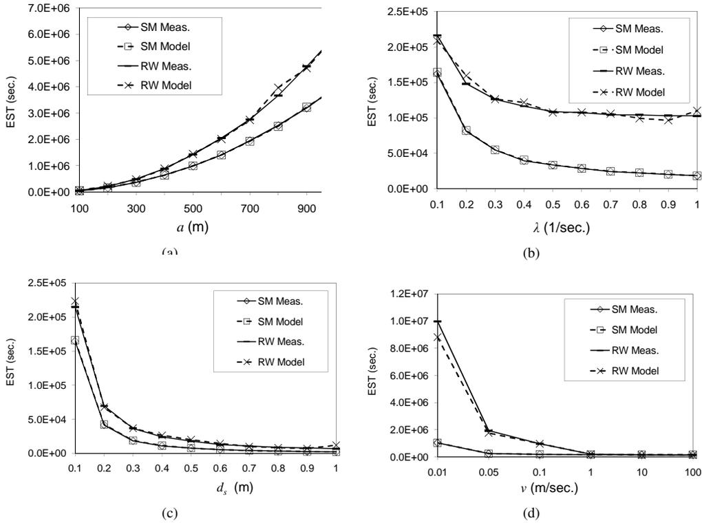
Fig. 5. Simulation results in (a), (b), (c), and (d) for validating Theorem 1 with respect to  $a$ ,  $\lambda$ ,  $d_s$ , and  $v$ , respectively. SM stands for the slap method. RW stands for the random walk. Model means the model prediction of the EST. Meas. means the measured mean searching time.
