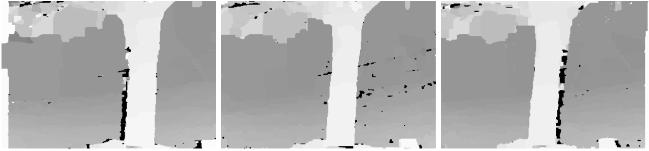
Figure 10: Effect of using the undefined label for 11-frame flower garden sequence (64 depth levels, no visibility terms, using best frames): (a) Reference image is 1st image, (b) Reference image is 6th image, (c) Reference image is 11th image. The undefined label is black, while the intensities for the rest are bumped up for visual clarity.
