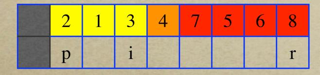
Select pivot (orange element) and rearrange: larger elements to the left of the pivot (red) elements not exceeding the pivot to the right (yellow)
