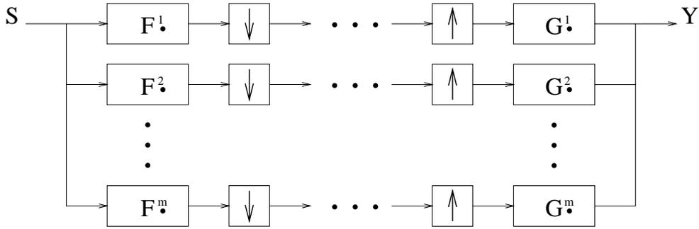
**Figure 2:** A filter bank for signals in the group ring  $AG$  with  $m$  channels.
