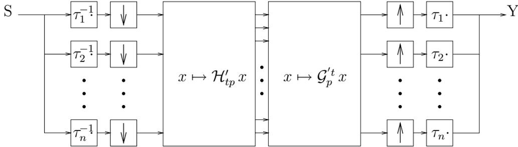
**Figure 3:** Polyphase implementation of a filter bank. The transpose of  $\mathcal{G}'_p$  is the left inverse of  $\mathcal{H}'_{tp}$  in a perfect reconstructing filter bank.
