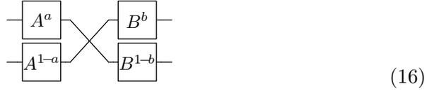
Clearly, this circuit is not able to realize a controlled- $U$  operation, because it cannot entangle any unentangled input state.  $\square$
