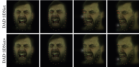
Figure 8. The error visualization of DAD-3DNet [34] and our DAD-3DNet+ on MultiFace [64] dataset. The white and green dots are the ground truth and predicted landmarks, respectively. We use the red line to show the error distance. From left to right, the head pose increases gradually.
