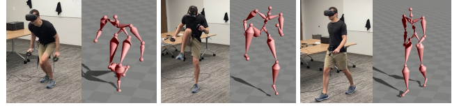
Figure 9: Pose prediction for real VR device. Our network is capable of generating difficult motions such as knee strikes or jumps.
