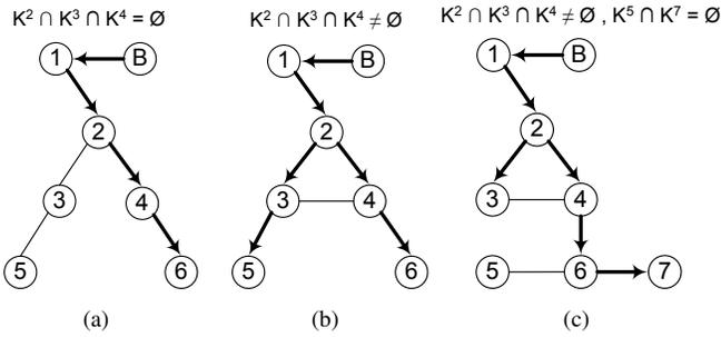
Fig. 2. Comparison of SFNK and HPP. a) There is no solution for SFNK or HPP, since node 2 has to choose either node 3 or node 4 as the next hop. b) SFNK has a solution because of the availability of a key shared by nodes 2, 3, and 4 that makes a triangle. c) There is no solution for SFNK and HPP, although the graph has a triangle.
