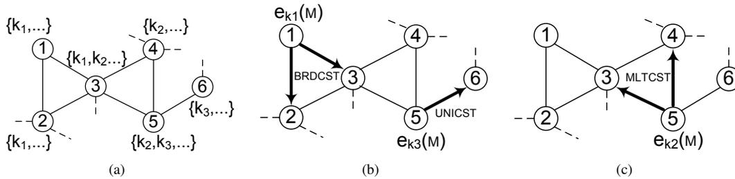
Fig. 1. Example of keys distributed by S-WGPS. a) Network connectivity and key distribution. b) The broadcast message sent by node 1 can be decrypted by all its neighbors (BRDCST) while only node 6 can decrypt the message sent by node 5 (UNICST). c) A subset of neighbors can decrypt the message sent by node 5 (MLTCSST).
