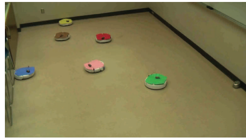
Fig. 7. Experimental setup consisting of 6 iRobot Creates equipped with Epic motes.
