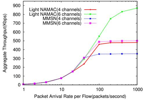
Figure 8: Aggregate Throughput vs. PAR in a single-hop Sensor Network
