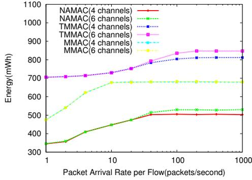
Figure 7: Energy consumption vs. PAR for a multi-hop Ad Hoc network
