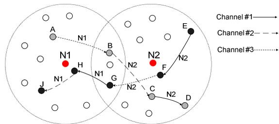
**Figure 1: Conceptual design for NAMAC. Nodes N1 and N2 act as negotiators for two data flows in the network: from A to D and from E to J. In this example, all nodes are equipped with radios with three channels. Each link is labeled with the ID of the negotiator responsible for that link. The arrow (i.e., continuous, dashed or dotted) represents the channel, decided by the respective negotiator, to be used by the nodes.**
