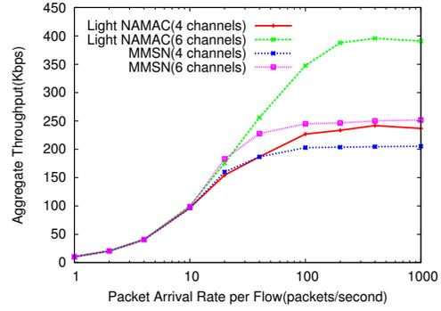
Figure 9: Aggregate Throughput vs. PAR in a multi-hop Sensor Network
