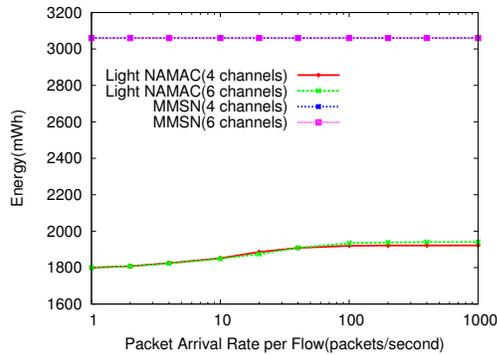
**Figure 11: Energy consumption vs. PAR for a multi-hop Sensor Network**
