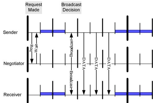
**Figure 3: Time slot and channel negotiation in Light-NAMAC. Protocol signaling and data communication are indicated by vertical arrows among Sender, Negotiator and Receiver. In this example, the Beacon Interval contains 3 Groups. Horizontal blue lines indicate time slots when a node sleeps.**
