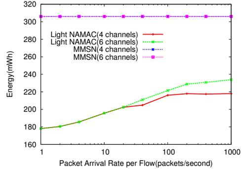
Figure 10: Energy consumption vs. PAR for a single-hop Sensor Network
