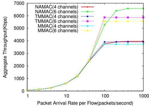
Figure 4: Aggregate Throughput vs. PAR in a single-hop Ad Hoc network
