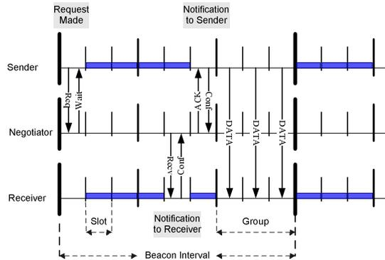
**Figure 2: Time slot and channel negotiation in NAMAC. Protocol signaling and data communication are indicated by vertical arrows among Sender, Negotiator and Receiver. In this example, the Beacon Interval contains 3 Groups. Horizontal blue lines indicate time slots when a node sleeps.**
