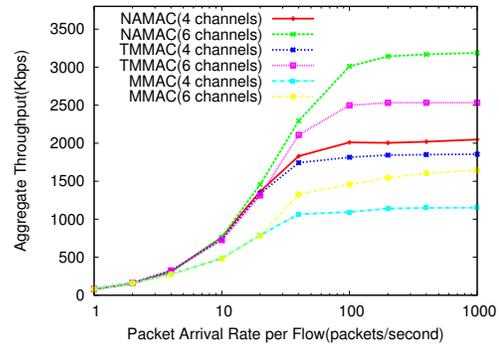
Figure 5: Aggregate Throughput vs. PAR in a multi-hop Ad Hoc network
