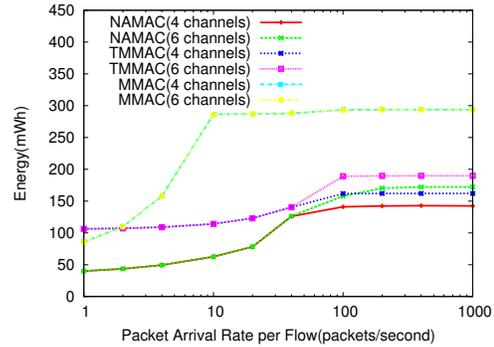
Figure 6: Energy consumption vs. PAR for a single-hop Ad Hoc network
