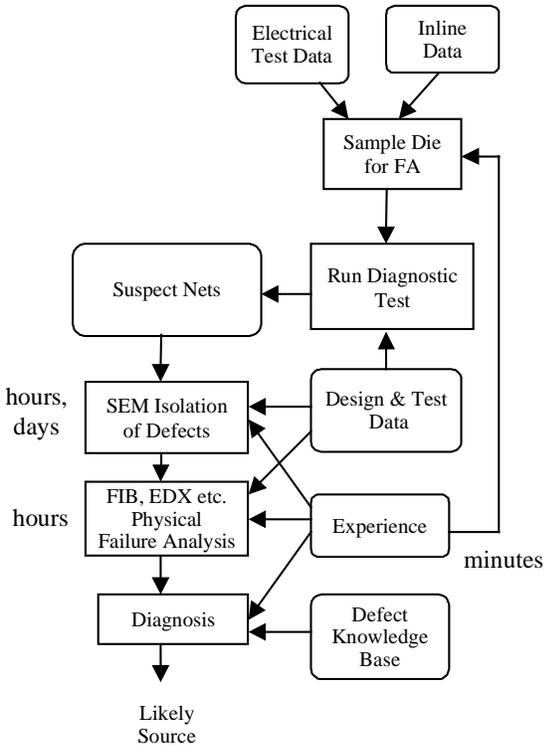
Figure 1. Current Defect Sourcing Approach
