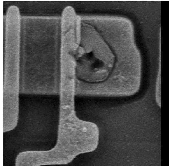
Figure 8. Close-up of gate-diffusion defect
