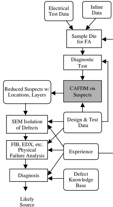
Figure 2. CAFDM modification of existing fault diagnosis approach
