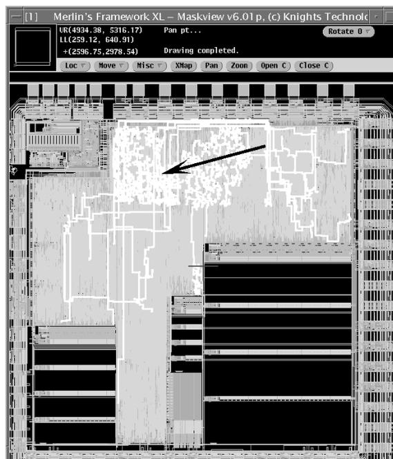
Figure 4. FIB3 potential bridging fault nets
