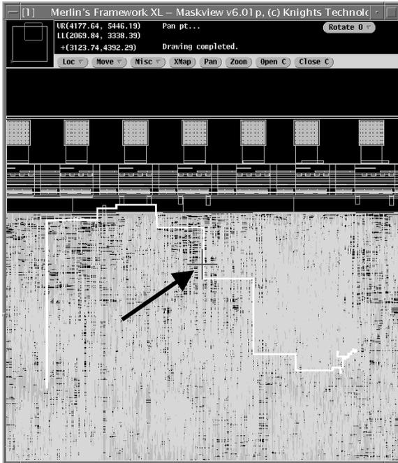
Figure 5. FIB3 CAFDM predicted and actual bridging fault location
