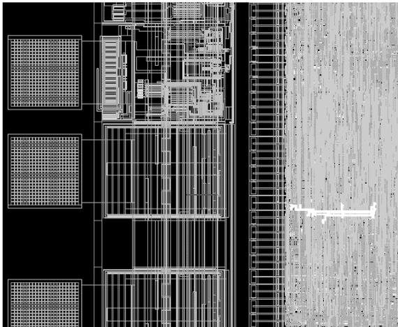
Figure 6. CHIP4 potential bridging fault nets
